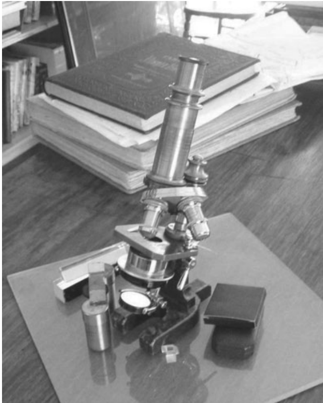
Figure 3. Microscope built by Ernst Goetz during his student days. Held by the Goetz family.
