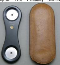
Bakelite handle. One mirror is condensing and the other is plane and both mirrors have a 4mm clear central sight hole. The instrument has a tan leather slip-in case.
