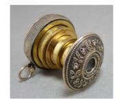
tiny artefact, only 15 mm long when closed and its 5 draw telescopic action extends it to 40 mm.
